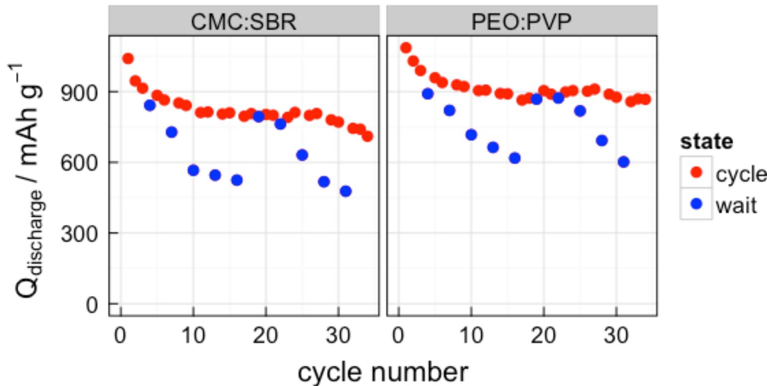
Self-discharge rate is roughly halved compared to CMC:SBR
