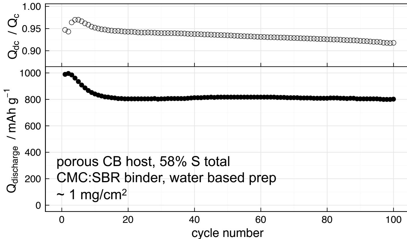
Electrolyte: 6  $\mu\text{L}/\text{mg}$  1 M LiTFSI, 0.25 M LiNO<sub>3</sub>, DME:DOL
