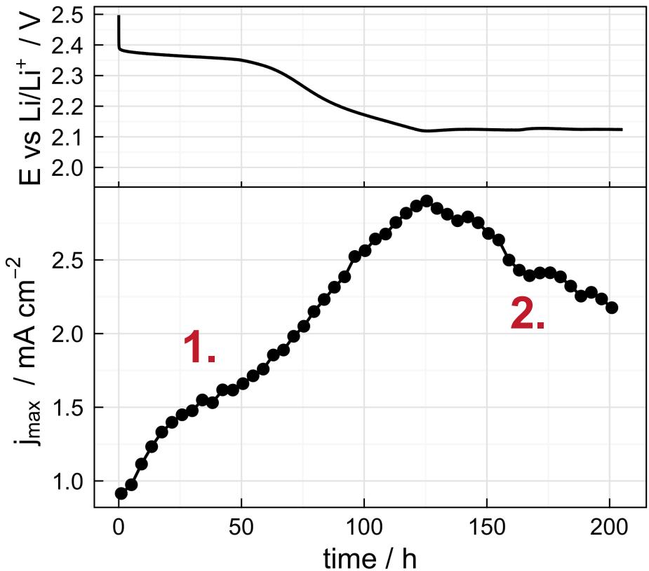
Redox shuttle drives S dissolution out of positive electrode.
