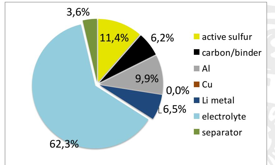
5  $\mu\text{L/mg}$ , 100% excess Li, no Cu c.c.,  $\sim 3 \text{ mAh/cm}^2$
